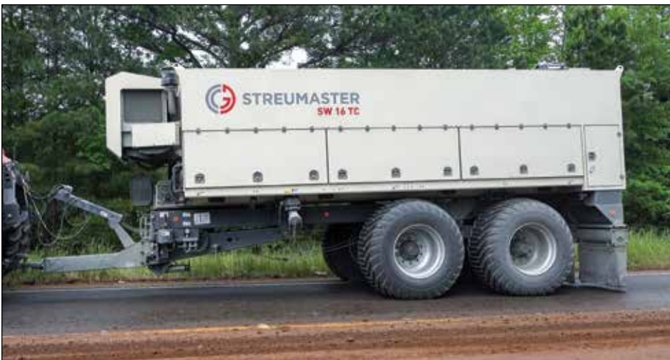
A Streumaster SW 16 cement spreader meters out dry cement during a road rehabilitation project.
