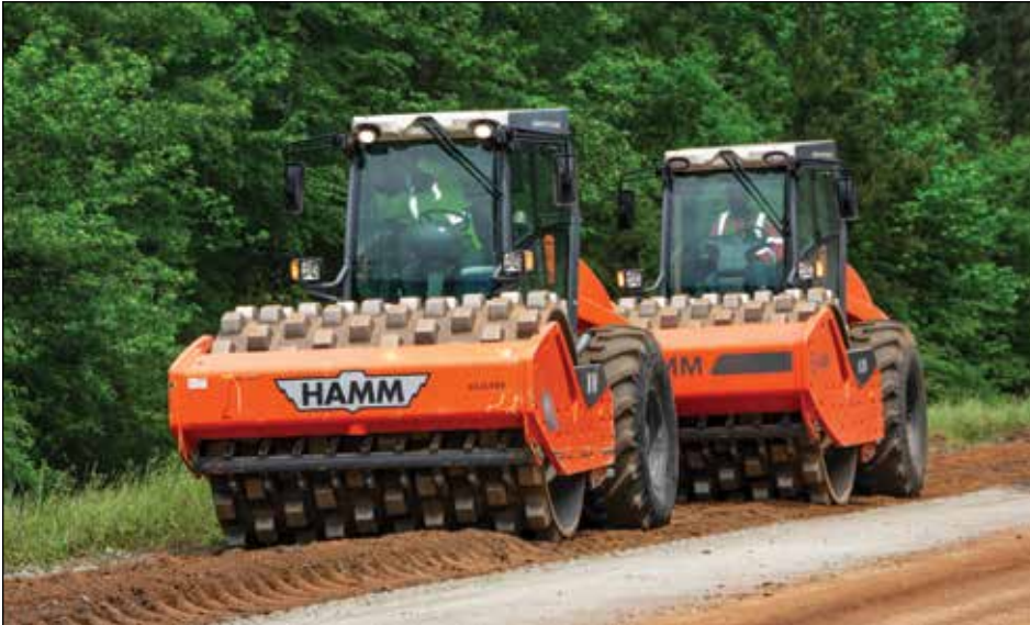
Compaction is done with Hamm rollers such as the H 16i P padfoot shown here, as well as smooth drum HD + 120i models.
