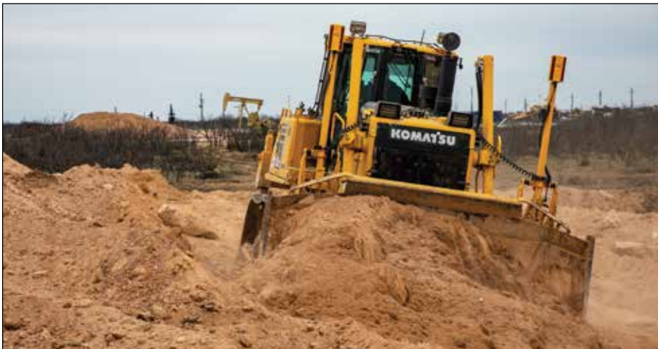
For general pushing, shaping and grading, Dorado Construction Group deploys Komatsu D85EX-18 dozers. The firm also uses Komatsu excavators and wheel loaders for various tasks. "The increases in productivity and efficiency we get across the board with Komatsu are fantastic," stated Fleet Manager/Equipment Manager Clay Butler.
