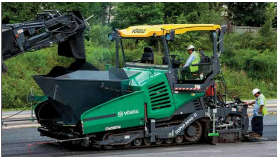
Kirby-Smith Machinery is working with a customer on a full-depth reclamation study that involves milling and replacement of asphalt pavements in lifts of six inches using a VÖGELE adjustable, high-density tamper bar screed on the VÖGELE Super 2000-3i paver.
