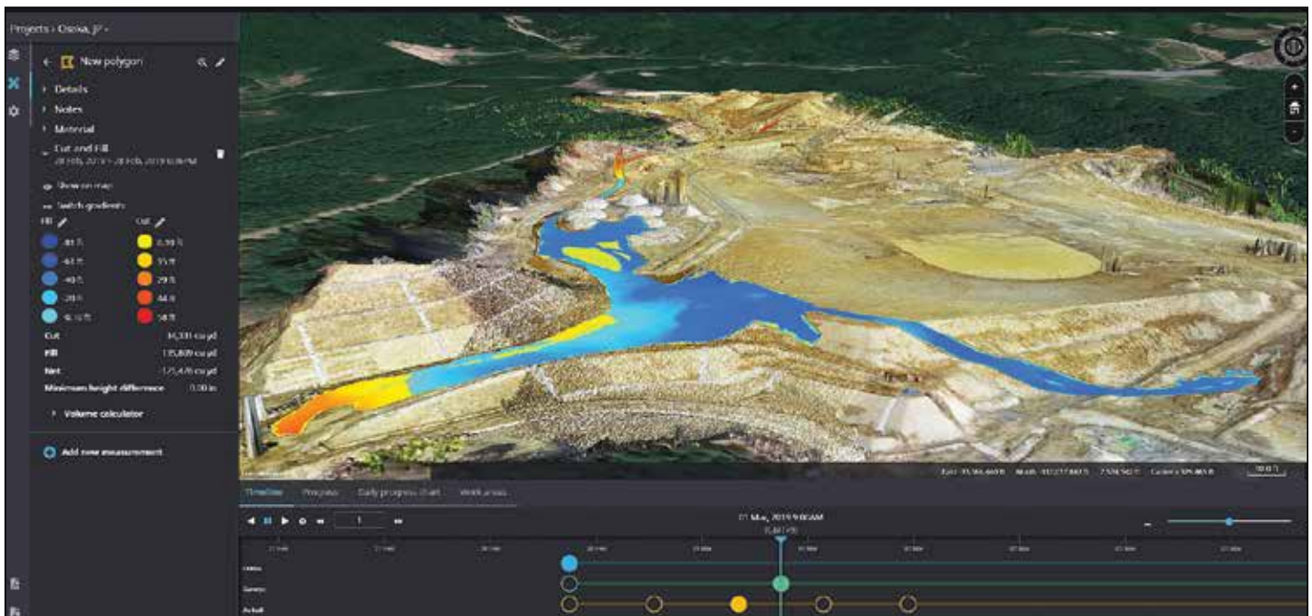
Smart Construction solutions include a dashboard that helps to visualize and analyze design, drone and machine as-built data to measure cut-fills, quantities and productivity.
