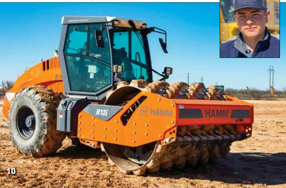
Brady Fenn compacts dirt on a pad site with a HAMM H 12i padfoot roller. "It has good visibility and is easy to run," said Fenn.
