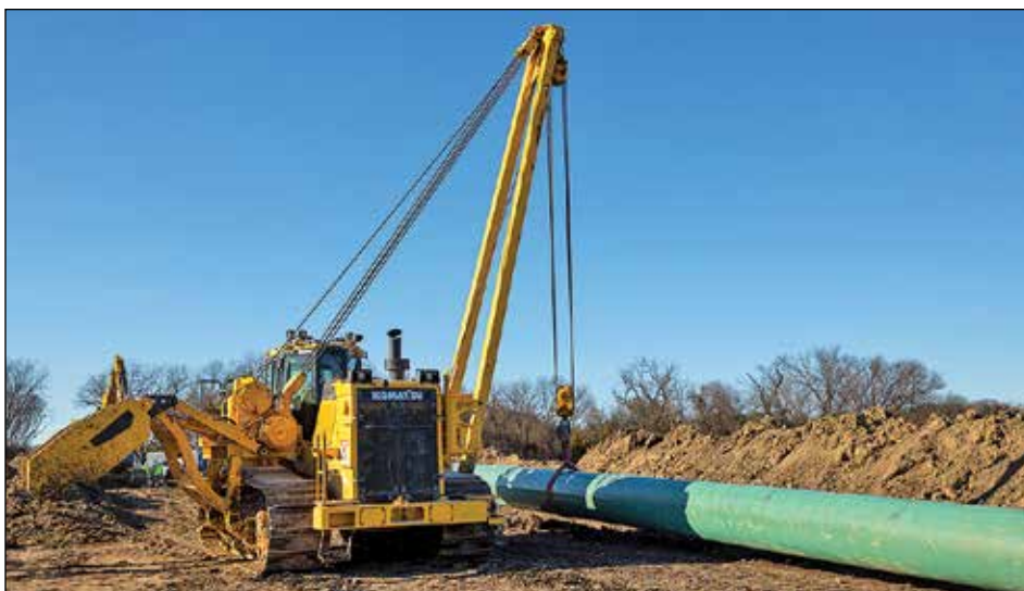
The new D155CX-8 pipelayer has an oval design nine-roller track that features 12 feet, 10 inches of track on ground for stability. With a 170,000-pound lift capacity, the D155CX-8 can handle up to 36-inch steel pipe. It offers a K170 pipelayer package with a standard 24-foot boom length.
