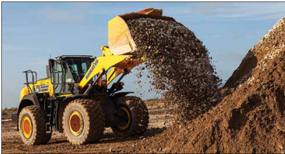
Komatsu incorporated next-generation technology with considerable benefits to make its new WA475-10 wheel loader an ideal fit for quarry, waste, infrastructure, forestry and non-residential applications. It's 30% more fuel efficient, has 18% greater horsepower, 20% more boom lift force and a breakout force increase of 8% compared to its predecessor model.
