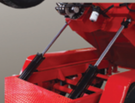
Dump System - Pivot Point & V-Body
