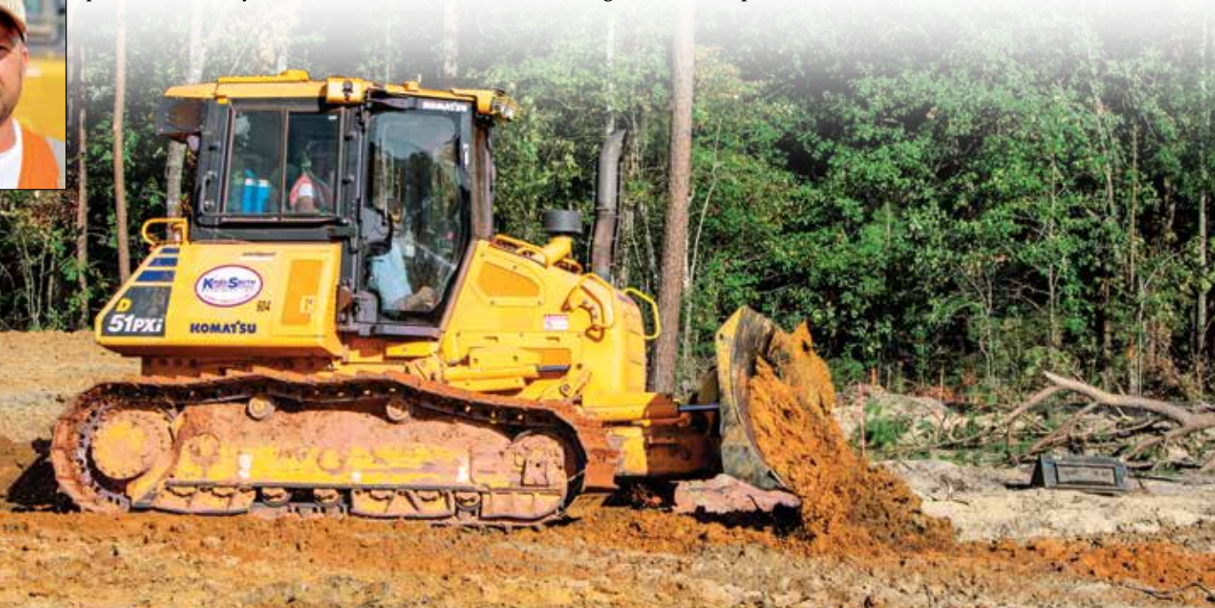
Operator Joshua Cooper cuts grade on a road project in Tyler, Texas, with a Komatsu D51PXi-24 iMC dozer. "The accuracy is spot-on, and it always knows where it is in relation to finished grade," said Cooper. "That saves us time and material costs."
