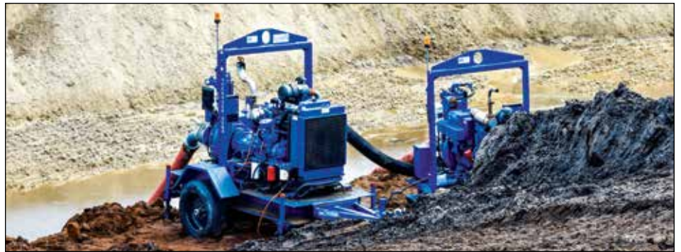
KSM now carries Thompson Pump heavy-duty, diesel-powered bypass and dewatering pumps throughout Oklahoma, North Texas and West Texas.
