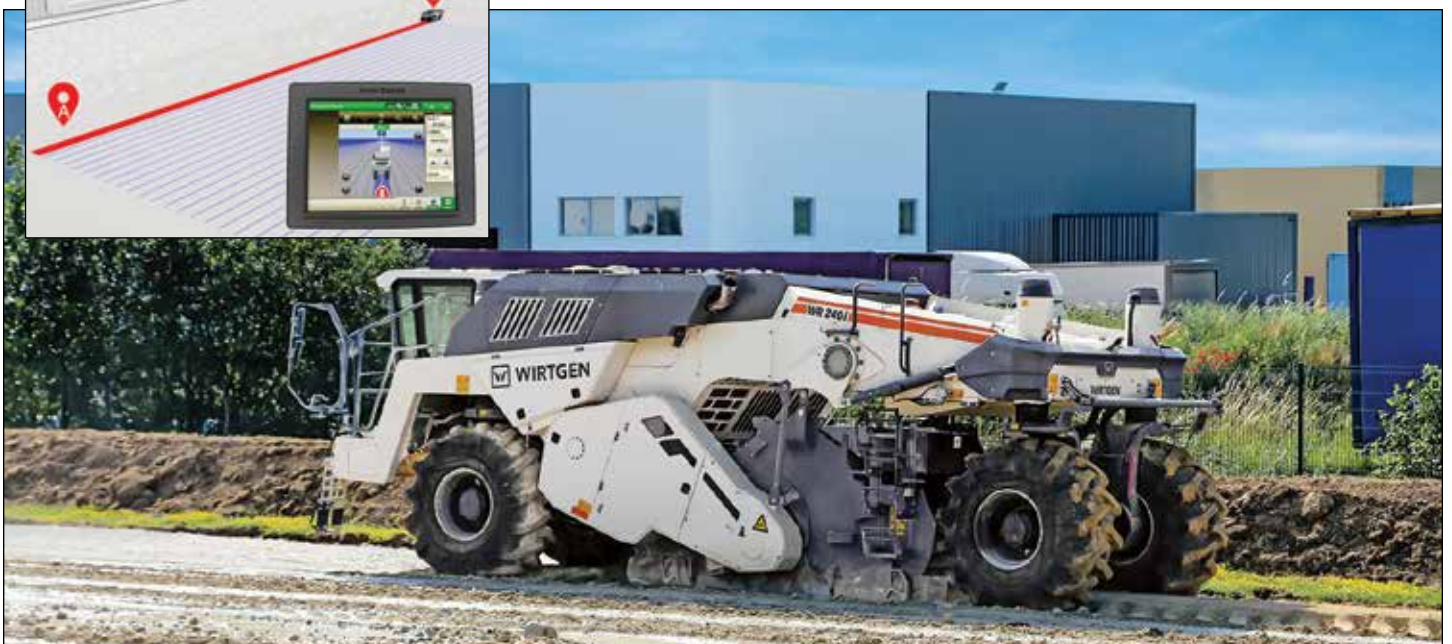
WIRTGEN's AutoTrac system for WR Series recyclers and stabilizers provides automatic steering for increased efficiency, resource conservation and reduced operator workload.
