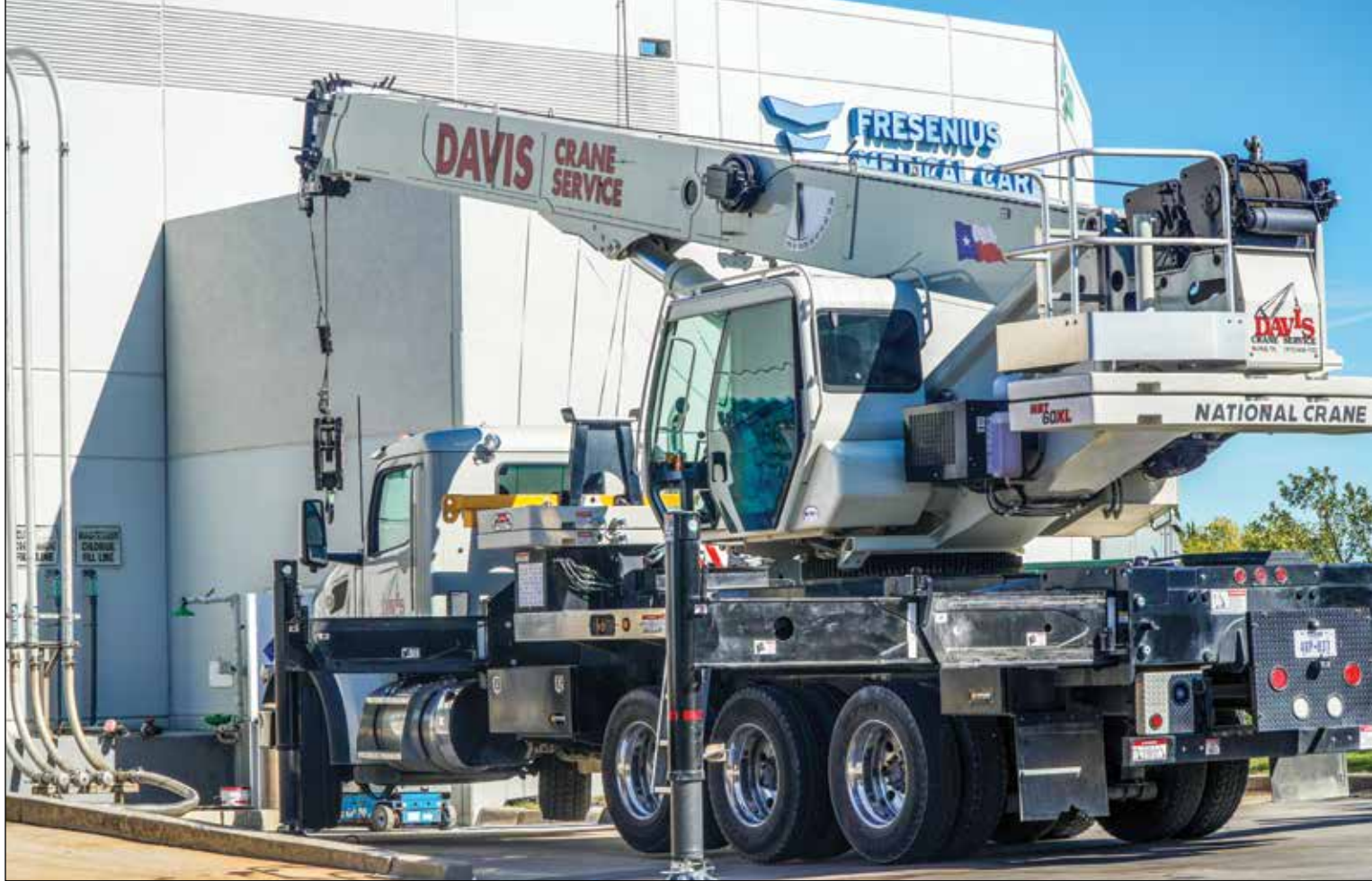
A Davis Crane Group operator lifts a tank part with a National Crane NBT60XL boom truck on a jobsite in the Dallas-Fort Worth area.
