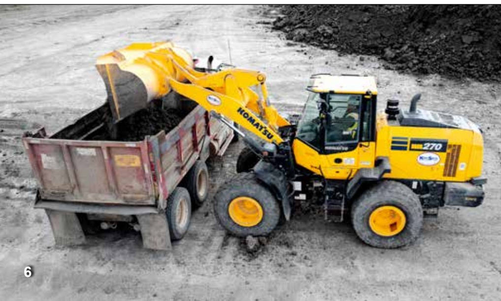
An L.A. Fuller and Sons operator loads trucks with a Komatsu WA270 wheel loader.
